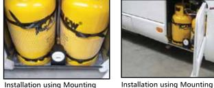
Installation using Mounting Bracket with a 0.6metre hose and right angle adaptor (01-4210)
