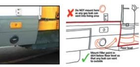
Fit in the skirt of the vehicle. below the floor level as any escaping gas can then vent freely to the atmosphere
