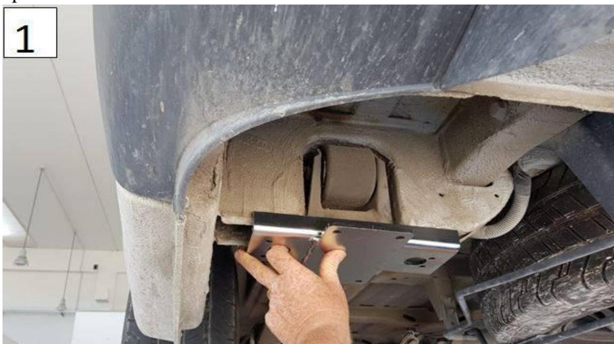
Put the adapter in the point illustrated, the rear support of the crossbow suspension Step 2:
