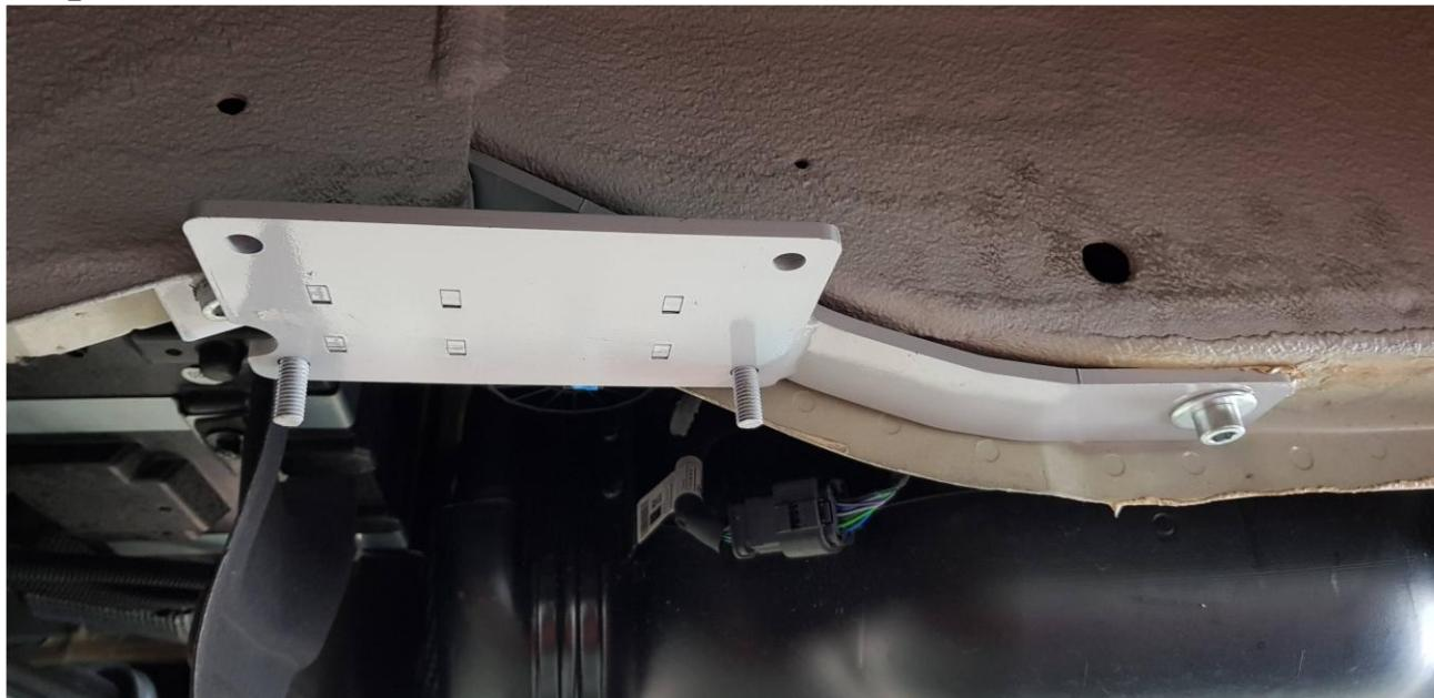
Fit the adapter with the bolts supplied
