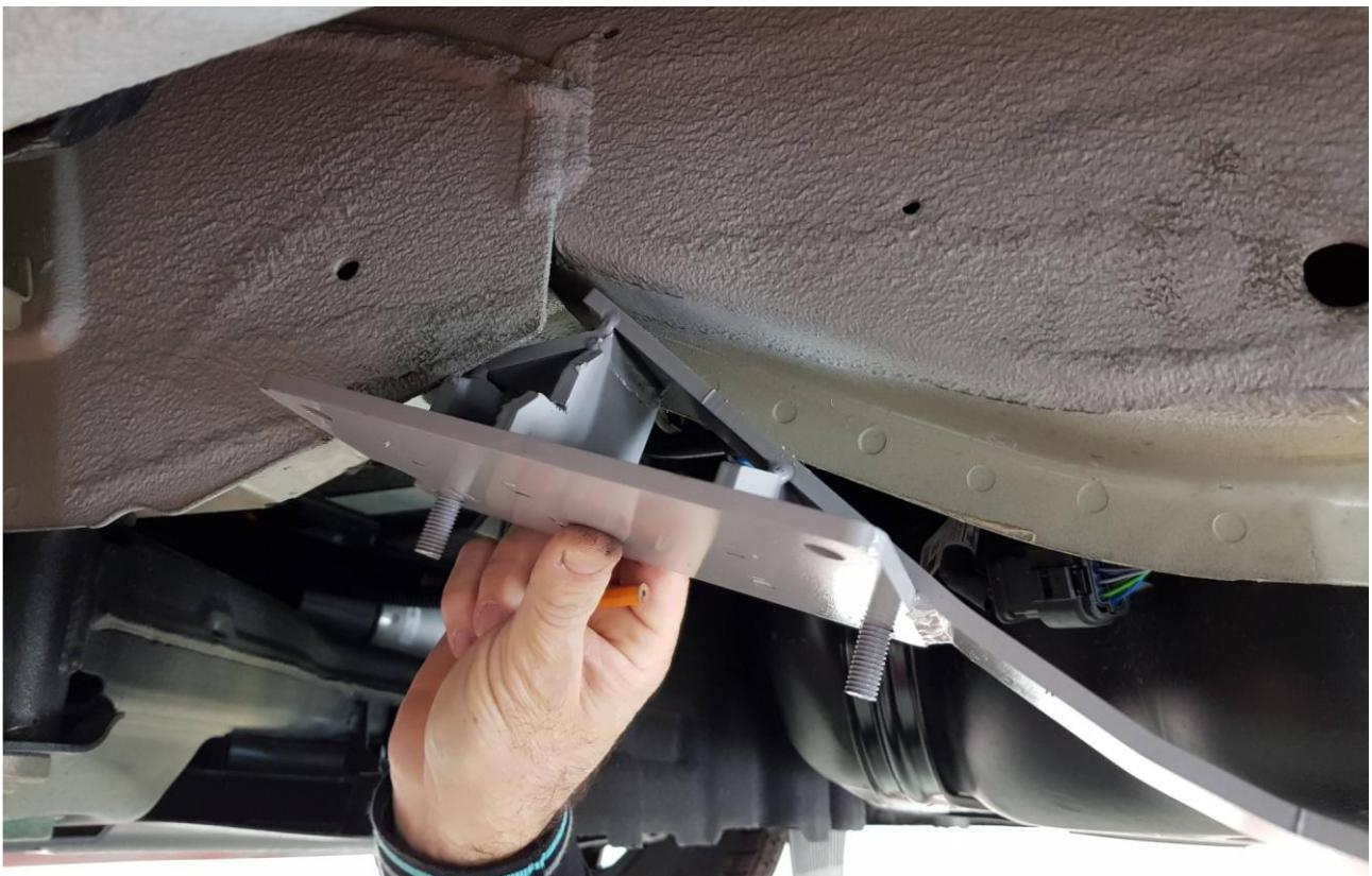
Insert the adapter in the space present on the chassis and push most frontly possible.
