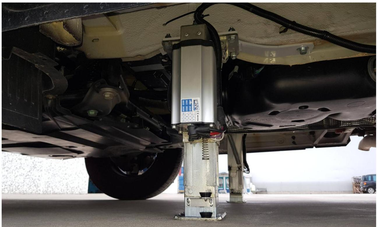
*EXAMPLES OF JACKS CORRECTLY INSTALLED*
